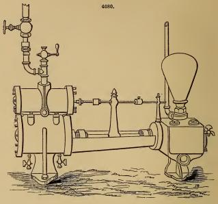
at pleasure; the pistons have a metallic packing, and there is a reservoir of air on the top of the water-cylinder, designed to regulate the ascension.
